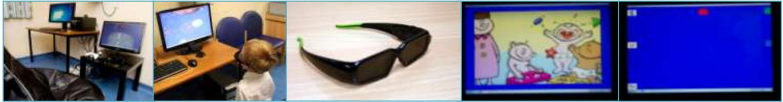
**Figure 1:** A: I-BiT™ kit including clinician and patient monitors B: Interactive video game. C: Shutter Glasses D: DVD footage as seen by left and right eye separately. Border images can be displayed to either eye.
